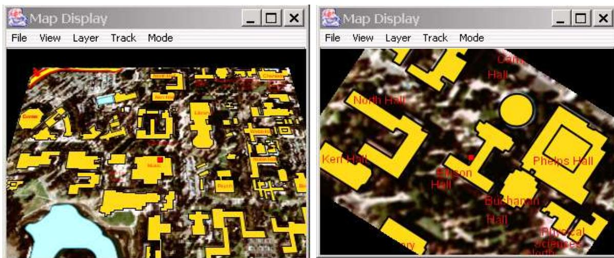
For different applications, and to facilitate usability studies, the system is designed to have alternative visualizations for the image and map data, and to allow the user choices. There are different factors that control how the geographic data are visualized upon the interface, which falls into two categories: dynamic signals, and user-controlled degrees of freedom. These are characterized as follows.
