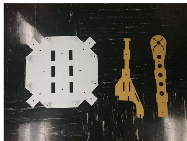
The three unique pieces of an early version of Symetrix-Wing unassembled.
