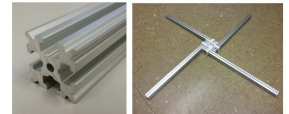
OpenBeam slotted aluminum extruded bar at left, with configuration of the new design at right.
