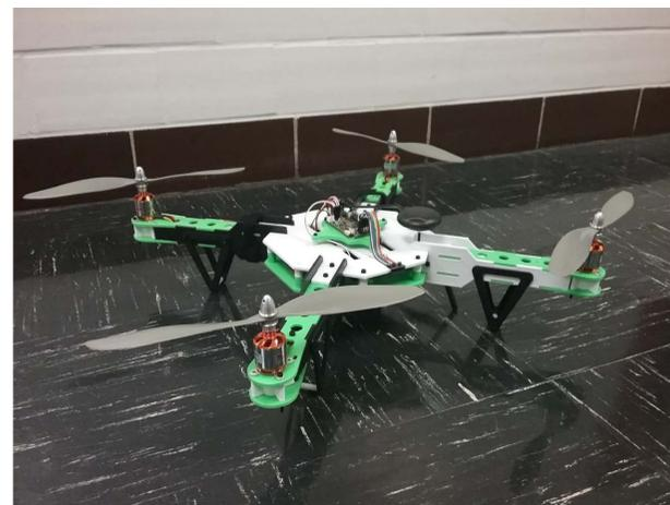
The fully assembled Symetrix-Wing with motors and flight controller.
